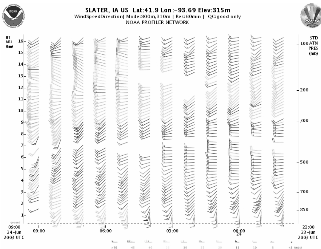
Figure 4.10 The Slater, IA 404 MHz Wind Profiler Plot. Time proceeds from right to left starting at 0000 UTC on 24 June and ending on 0900 UTC on 24 June. The profiler is located 86 km south of the MIPS location. A full barb represents 10 \text{ m s}^{-1} .
